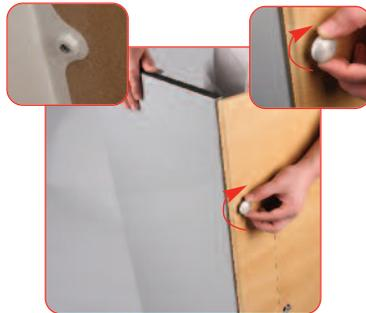
To build the base of the unit align front with the locators on the sides, Screw the turn parts through the front and into the side panel. Repeat this for the remaining sides
